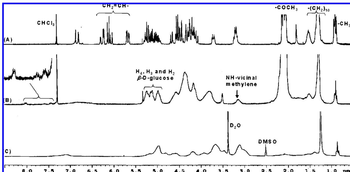
**Figure 1.**  $^1\text{H}$  NMR spectra of (A) monomer **B'** (in  $\text{CDCl}_3$ ), (B) acetylated NA20-78 (in  $\text{CDCl}_3$ ), and (C) deprotected NA20-78 (in  $\text{DMSO}-d_6$ ).
