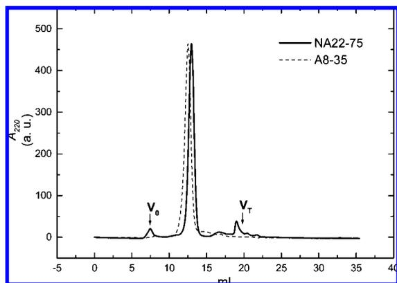
**Figure 3.** ASEC of NAPols NA22-75 and A8-35 on a Superose 12 10-300 GL column (Tris-HCl 20 mM, NaCl 100 mM, pH = 8.5) at 20 °C. The two polymers were detected by their absorbance at 220 nm, and the chromatograms were normalized to the same maximum.
