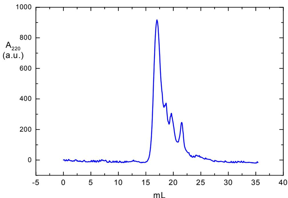
**Figure S9.** SEC chromatograms of impurities separated from NA20-79 during dialysis (Superose 12 10-300GL column, elution with Tris buffer ([Tris-HCl/Tris] = 20 mM, [NaCl] = 100 mM, pH = 8.5), detection at 220 nm). 16 mg of the exterior dialyzed materials were put in suspension in 500  $\mu$ L of mQ water. The suspension was stirred for 1 day and centrifuged. The supernatant was taken off and injected on a Superose 10-300GL column.
