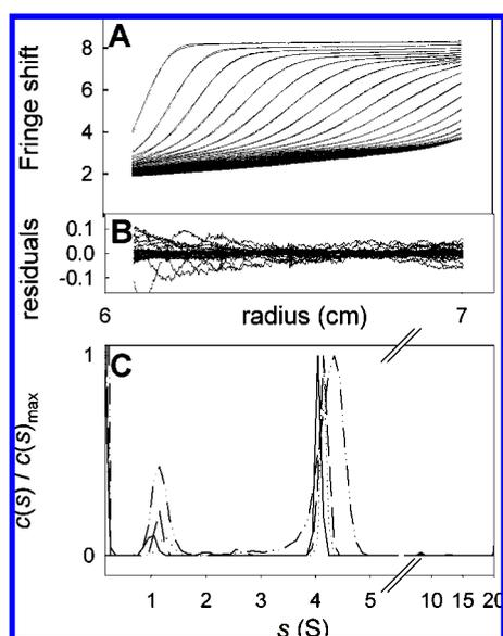
**Figure 4.** SV analysis of NA20-78. (A) Superimposition of selected experimental and modeled SV profiles obtained over 11 h at 42 000 rpm and 20 °C, using interference optics, for water-solubilized NA20-78 at 2.5 g·L<sup>-1</sup>. (B) Corresponding residuals. (C) Superimposition of the  $c(s)$  distributions obtained for NA20-78 at 9.81 (solid line), 5.13 (long dash), 2.44 (dotted) and 0.95 (dash-dot-dot) g·L<sup>-1</sup>. For clarity, the  $c(s)$  scale is normalized to a maximum value of 1.
