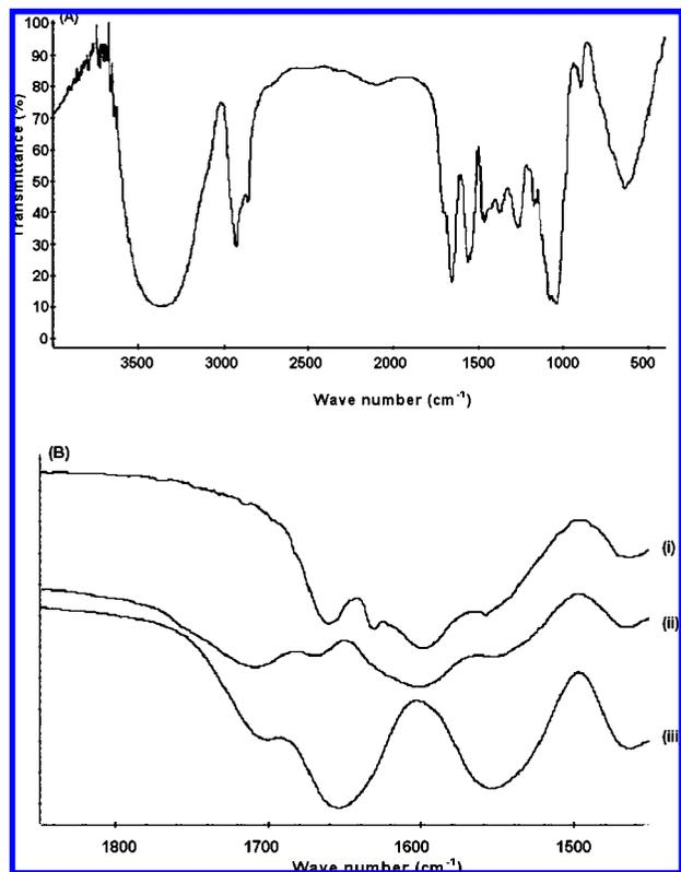
**Figure 2.** Fourier transform infrared (FTIR) spectra of (A) deprotected NA25-78, from wavenumber 400  $\text{cm}^{-1}$  to 4000  $\text{cm}^{-1}$  and (B) (i) deprotected monomer **A**, (ii) deprotected monomer **B**, and (iii) NA25-78, from wavenumber 1400  $\text{cm}^{-1}$  to 1800  $\text{cm}^{-1}$ .
