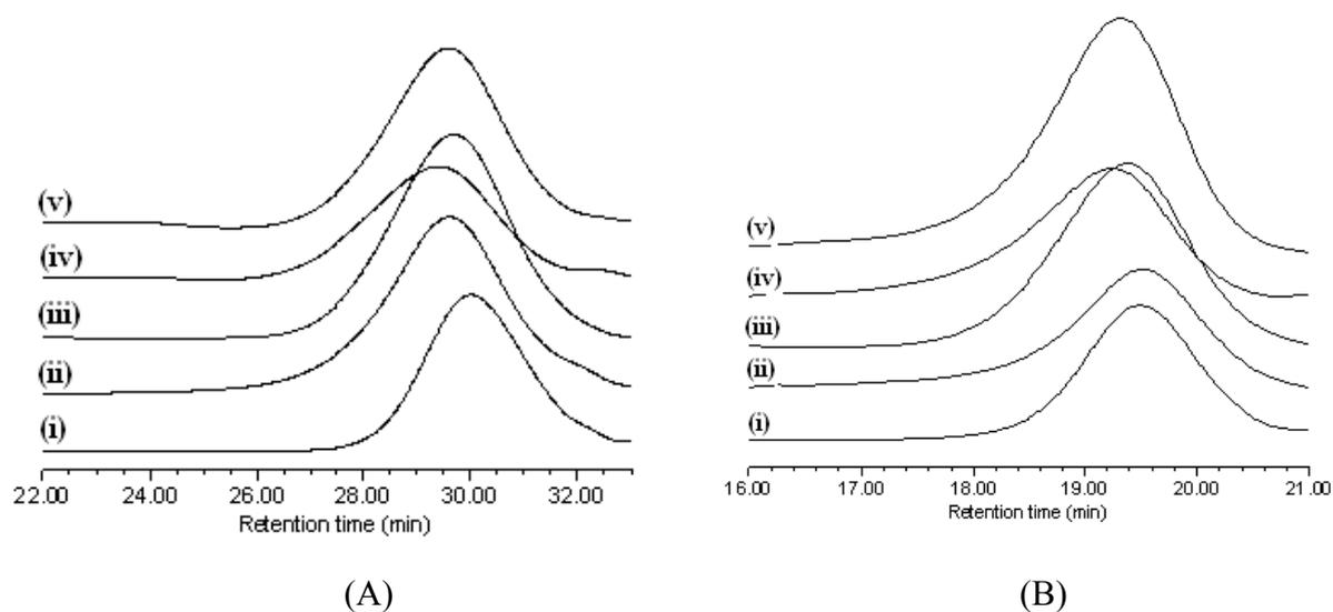
**Figure S4.** GPC traces of different cotelomers using (A) THF + 0.1% TFA, (B) DMF: (i) NA22-83, (ii) NA22-75, (iii) NA20-78, (iv) NA29-83, (v) NA25-78.
