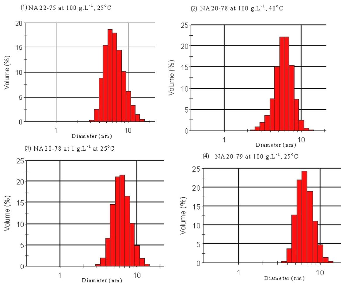
**Figure S7.** Hydrodynamic diameter distribution statistical plot (by volume) of different NAPols from DLS.
