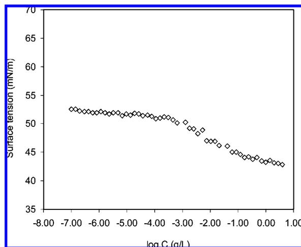
**Figure 5.** Evolution of the surface tension of aqueous solutions of NA20-78 as a function of concentration at 20 °C.
