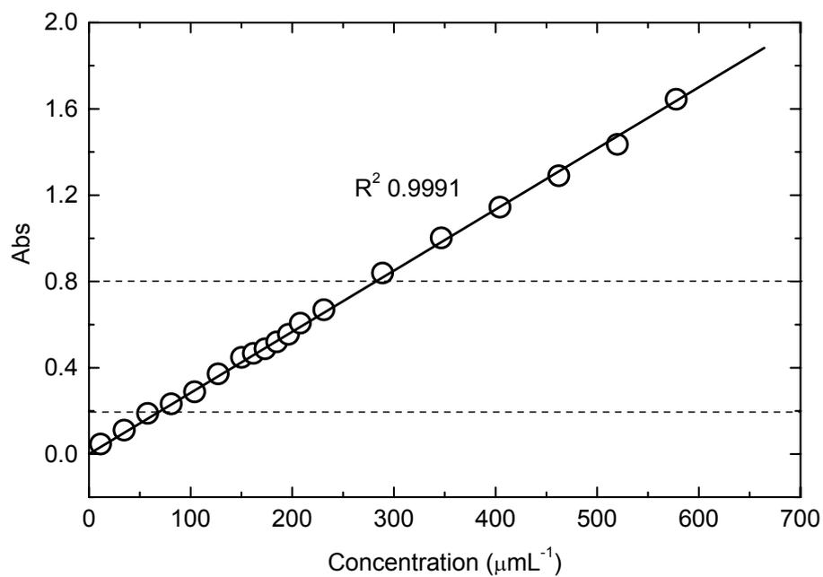
**Figure S3.** UV calibration curve of telogen agent (**2**) (at  $\lambda_{\max} = 272$  nm, 25°C).
