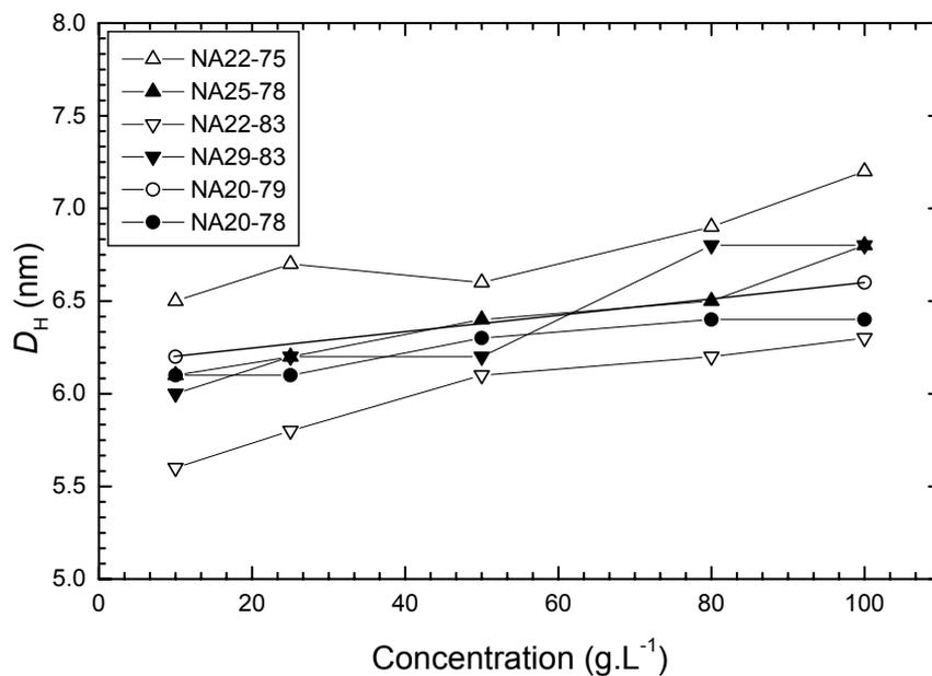
**Figure S6.** Evolution as a function of concentration of the hydrodynamic diameter of the particles formed by different NAPols at  $25^{\circ}\text{C}$  in water, as measured by DLS.
