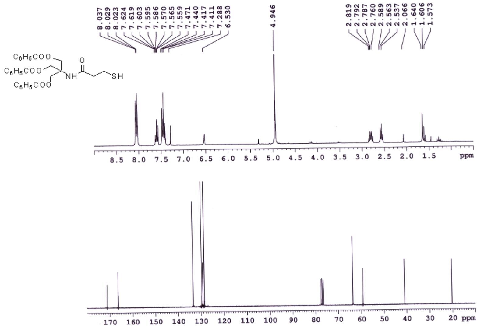
**Figure S1.** <sup>1</sup>H and <sup>13</sup>C NMR spectrum of telogen agent (2) in CDCl<sub>3</sub>.
