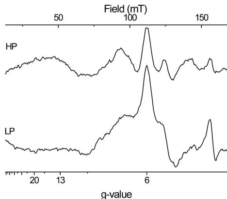
**Fig. 6.** Difference spectra of HP and LP components. Redox-induced EPR difference spectra of the high-spin heme signals of the isolated  $b_6f$  complex from *C. reinhardtii* are shown: HP, +362/+18 mV; LP, +18/−104 mV. EPR settings are as for Fig. 1.
