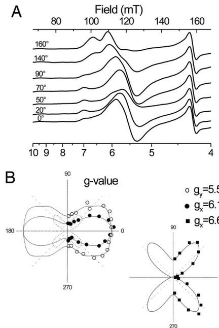
**Fig. 5.** Orientation of  $c_1$ 's  $g$  tensor in the presence of NQNO. (A) EPR spectra were recorded on partially ordered multilayers of chloroplast membranes from spinach in the presence of NQNO. The angle between the magnetic field and the membrane plane is indicated for each spectrum. EPR settings are as for Fig. 1 except for temperature ( $6$  K) and microwave power ( $63.8$  mW). (B) Polar plots of signal amplitudes are shown.
